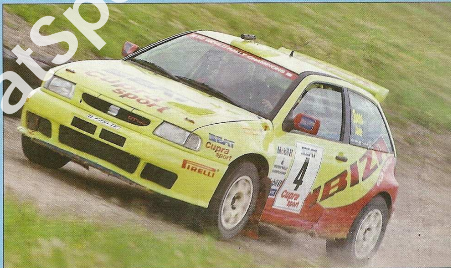
Second evolution of the Ibiza Kit Car proved to have a particularly well-sorted chassis – even when its wheels aren't connected to the ground. Body attrition is from Scottish Rally – car came straight from Scotland to the CCC test at the Silverstone RallySprint track
